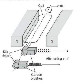
> Instantaneous value of emf produced by AC generator is given by  $e = NBA \omega \sin \omega t$ where, N = number of turns in the coil, B = strength of magnetic field, A =area of each turn of the coil  $\omega$  = angular velocity of rotation of coil.
