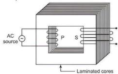
Working: When an alternating current is passed through the primary coil, the magnetic flux through the iron core changes, which does two things, produces emf in the primary coil and an induced emf is set-up in the secondary coil. If we assume that the resistance of primary coil is negligible, then the back emf will be equal to the voltage applied to the primary coil.
