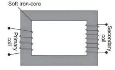
**Working:** When an alternating voltage is applied to the primary, the resulting current produces an alternating magnetic flux which links the secondary coil and induces an emf.
