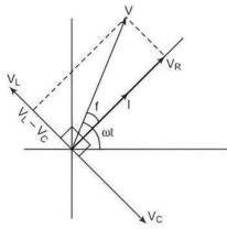
As it is evident from the figure,  $\overrightarrow{V_L}$  and  $\overrightarrow{V_C}$  are in opposite direction. Hence, their resultant will be  $(\overrightarrow{V_L}-\overrightarrow{V_C})$ . Using the law of parallelogram,  $\overrightarrow{V_R}$  and  $(\overrightarrow{V_L}-\overrightarrow{V_C})$  resultant is equal to the applied emf  $\overrightarrow{e}$  as given by the diagonal of the parallelogram.
