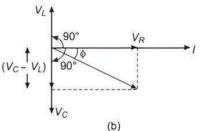
Suppose the voltage across resistance R is  $V_R$  voltage across inductance L is  $V_L$  and voltage across capacitance C is  $V_C$ . The voltage  $V_R$  and current i
