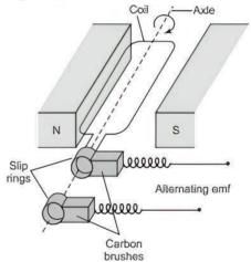
Let N be the number of turns in the coil. A be the area of face of each arm. B be the magnitude of the magnetic field.  $\theta$  be the angle which normal to the coil makes with field B at any instant t and  $\omega$  is the angular velocity with which coil rotates.
