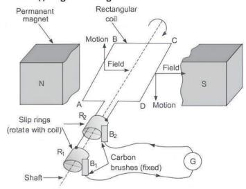
Let N be the number of turns in the coil, A be the area of face of each arm. B be the magnitude of the magnetic field,  $\theta$  be the angle which normal to the coil makes with field  $\overrightarrow{B}$  at any instant t and  $\omega$  is the angular velocity with which coil rotates.
